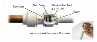
Like our Standard Fittings, Twist & Lock Fittings have a collet with stainless steel teeth that grip the pipe when fully inserted, and an O-ring to provide a permanent leak-proof seal. The additional benefit of the Twist & Lock Fitting is that a twist of the screw-cap gives greater compression on the O-ring seal and locks the pipe in place for greater security.
